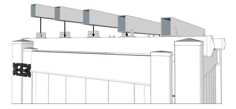
7. Secure Pergola Rails to Mounting Clips with screws provided.
