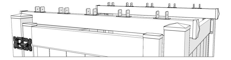
5. Secure Mounting Clips to Mounting Rails with Mounting Rail Screws provided.
