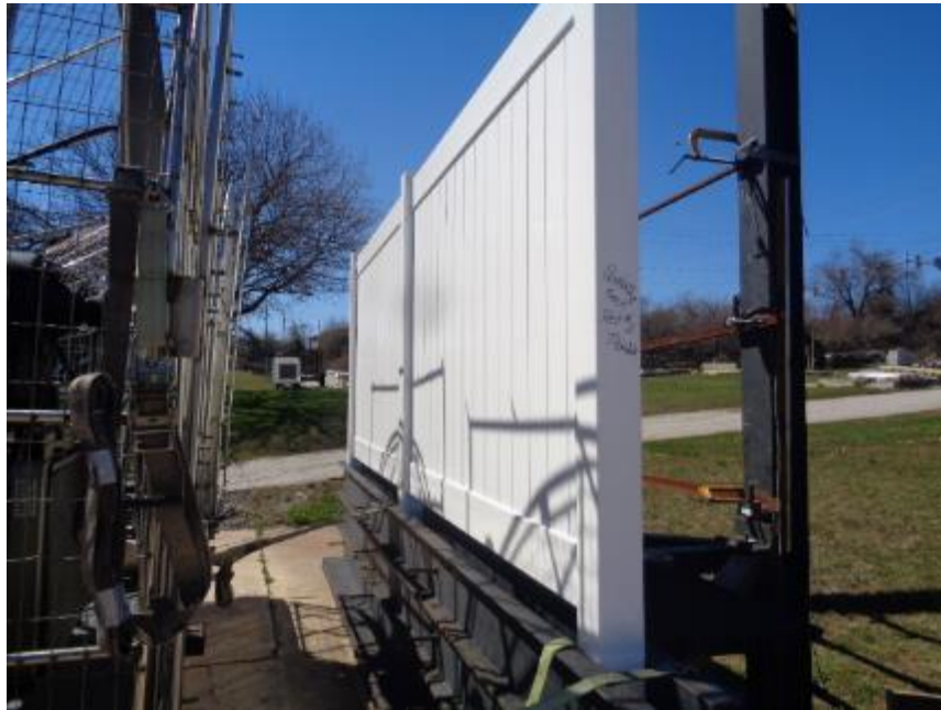
Photo No. 1 Typical Dynamic Wind Test Setup
