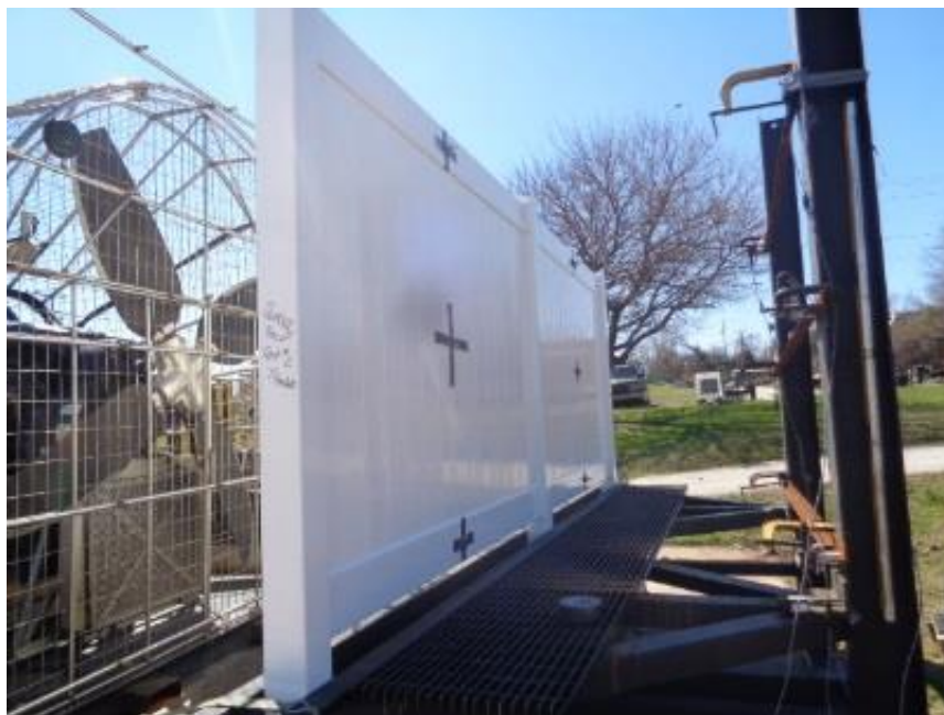
Photo No. 2 Transducer Locations on Backside of Fence Panels
