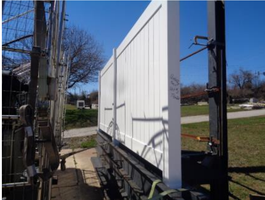
Photo No. 1 Typical Dynamic Wind Test Setup
